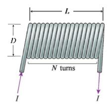
A1. (1 point) Assuming *I* is a positive number, what is the direction of the magnetic field at the centre of the solenoid? [Circle the best choice from the following six possibilities:]
