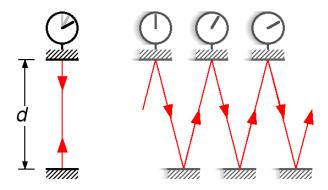
A short pulse of light bounces between the mirrors, "ticking" for each bounce.
