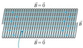
The magnetic field is uniform inside this section of an ideal, infinitely long solenoid. The magnetic field outside the solenoid is zero.
