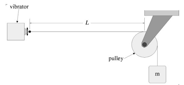
An object of mass, m=16 kg is hung from a string, which passes over a light, frictionless pulley. The other end of the string is connected to a vibrator, which sends waves along the string with a constant frequency, f. It has been found that 20 metres of this kind of string, when coiled up and placed on a scale, has a mass of 40 grams. The distance between the point where the string is tied to the vibrator and the point where the string touches the pulley is L=2.0 m.
