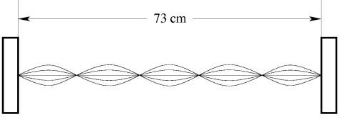
A standing wave is set up on a single string, as shown above. The two fixed ends are attached to walls 73 cm apart. The string is represented at several times.
