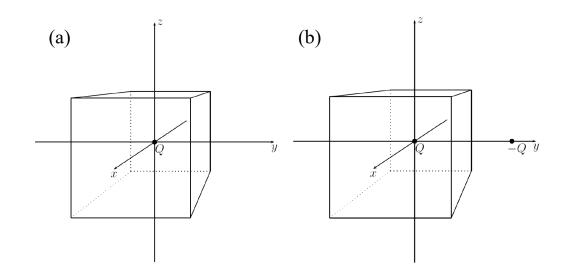
(b) A second charge, -Q, is now added at  $\vec{r} = (0, a, 0)$ , as shown on the right. Now what is the total flux through the box, and the average of the perpendicular component,  $E_{\perp}$ , on the face centred on (0, a/2, 0)?
