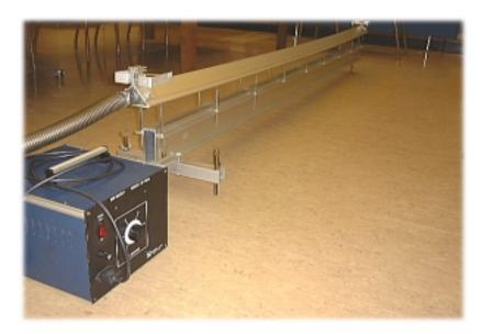
This experiment is an adaptation of **The AIR TRACK** to simple harmonic motion. This air track is shaped as an arc of a circle of large radius in the vertical plane. Thus a glider on the track behaves like the bob of a simple pendulum of large radius and thus long period. This enables simple harmonic motion to be "slowed down" for more leisurely observation.
