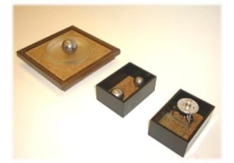
On first glance the motions of a sphere on a concave spherical surface of radius of curvature R might appear to be that of a simple pendulum of length R. However, a quick recognition of the effects of the moment of inertia of the sphere leads to a different conclusion. If a sphere of radius a undergoes small oscillations on a surface of radius R, without slipping, the period is given by:
