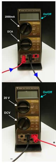
The upper knob controls the scale of the readings, and should be set to the shown **20V** position.
