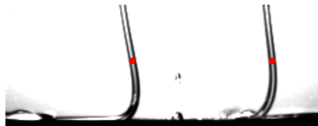
FIG. 5: Centres of strands, as detected by the algorithm
