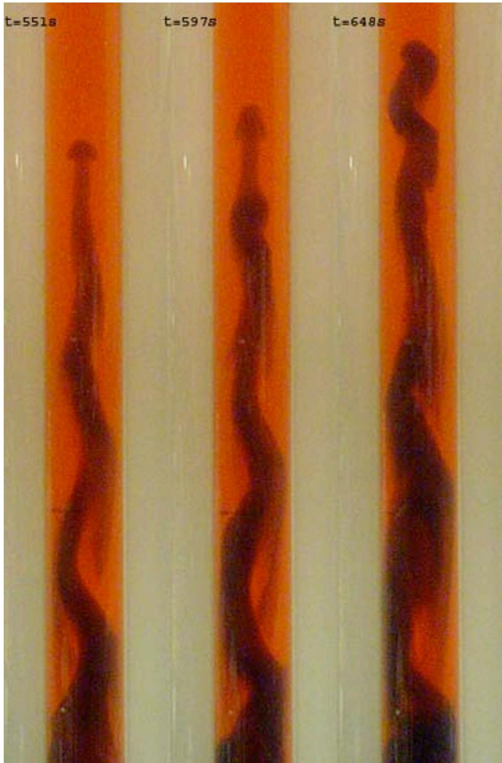
**Figure 3.3:** Three pictures for an experimental run at 20.00 °C detailing the snowballing of the lower part of a plume that eventually engulfs the plume head. The same 30 cm length of the tube is shown in each picture.
