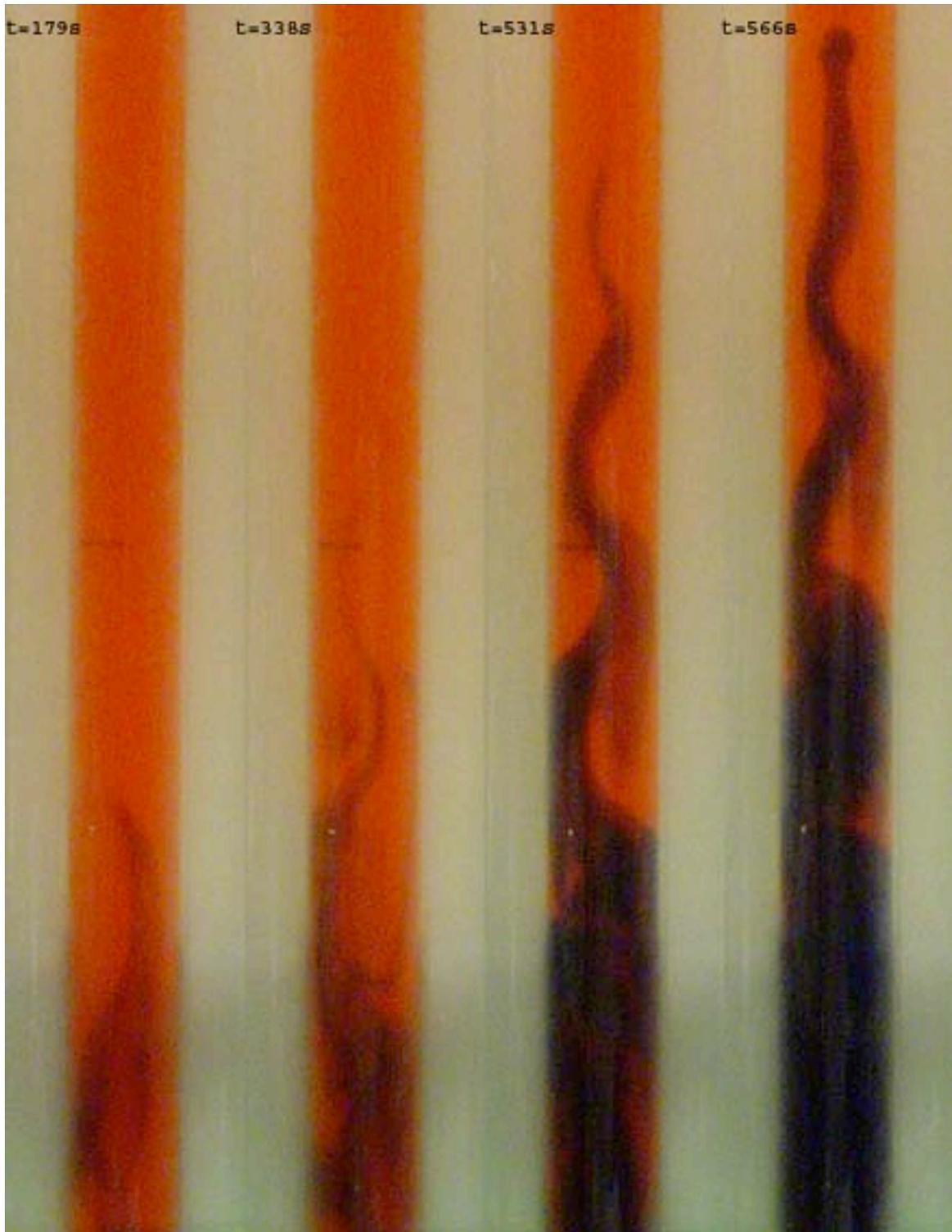
**Figure 3.2:** Four pictures for an experimental run at 12.50 °C detailing the transition between writhing to relatively straight vertical plume motion. The same 30 cm length of the tube is shown in each picture. At ~556s writhing motion has given way to straight rising.
