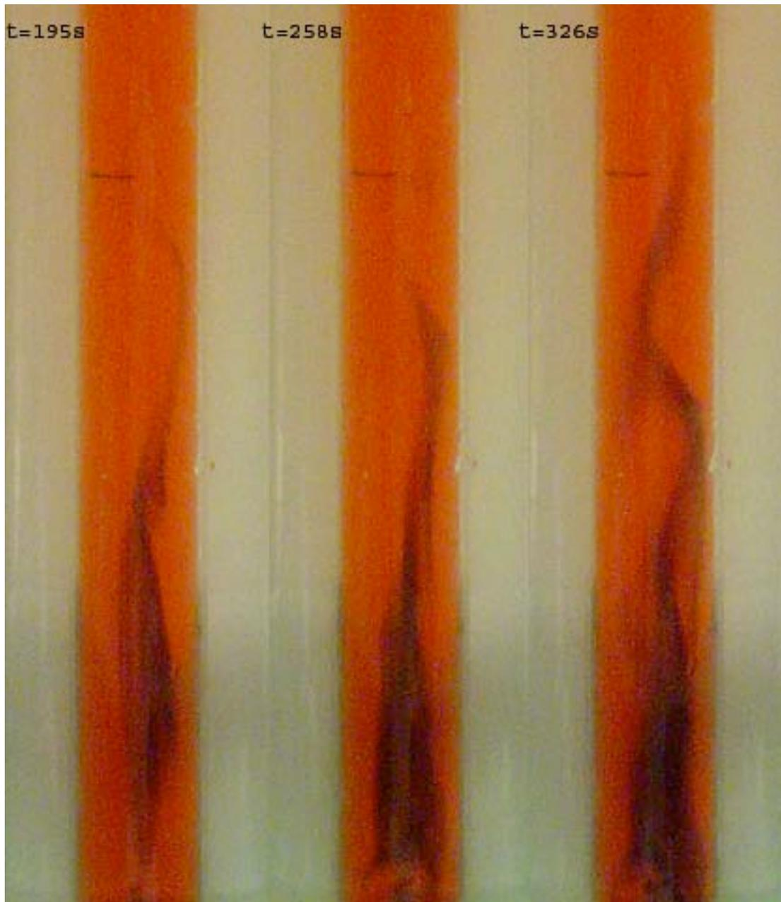
**Figure 3.4:** Three pictures for an experimental run at 12.50 °C detailing the collapse of a front filament. The same 28 cm length of the tube is shown in each picture.
