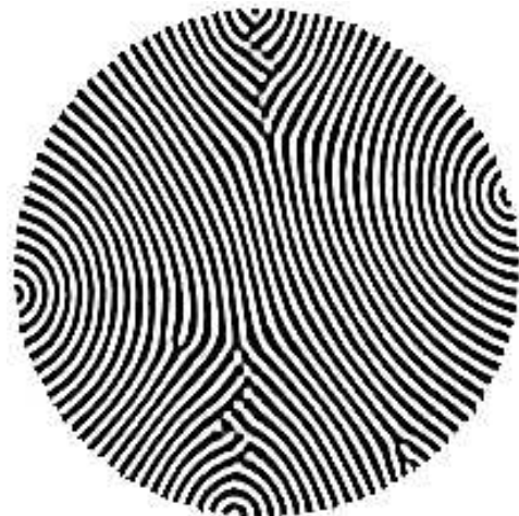
FIG. 4. An example of the curved rolls which appear in the Boussinesq case in a cell with \Gamma = 41 and for \sigma \simeq 1 when \epsilon is increased, in this case to 0.34. After Ref. [35].
