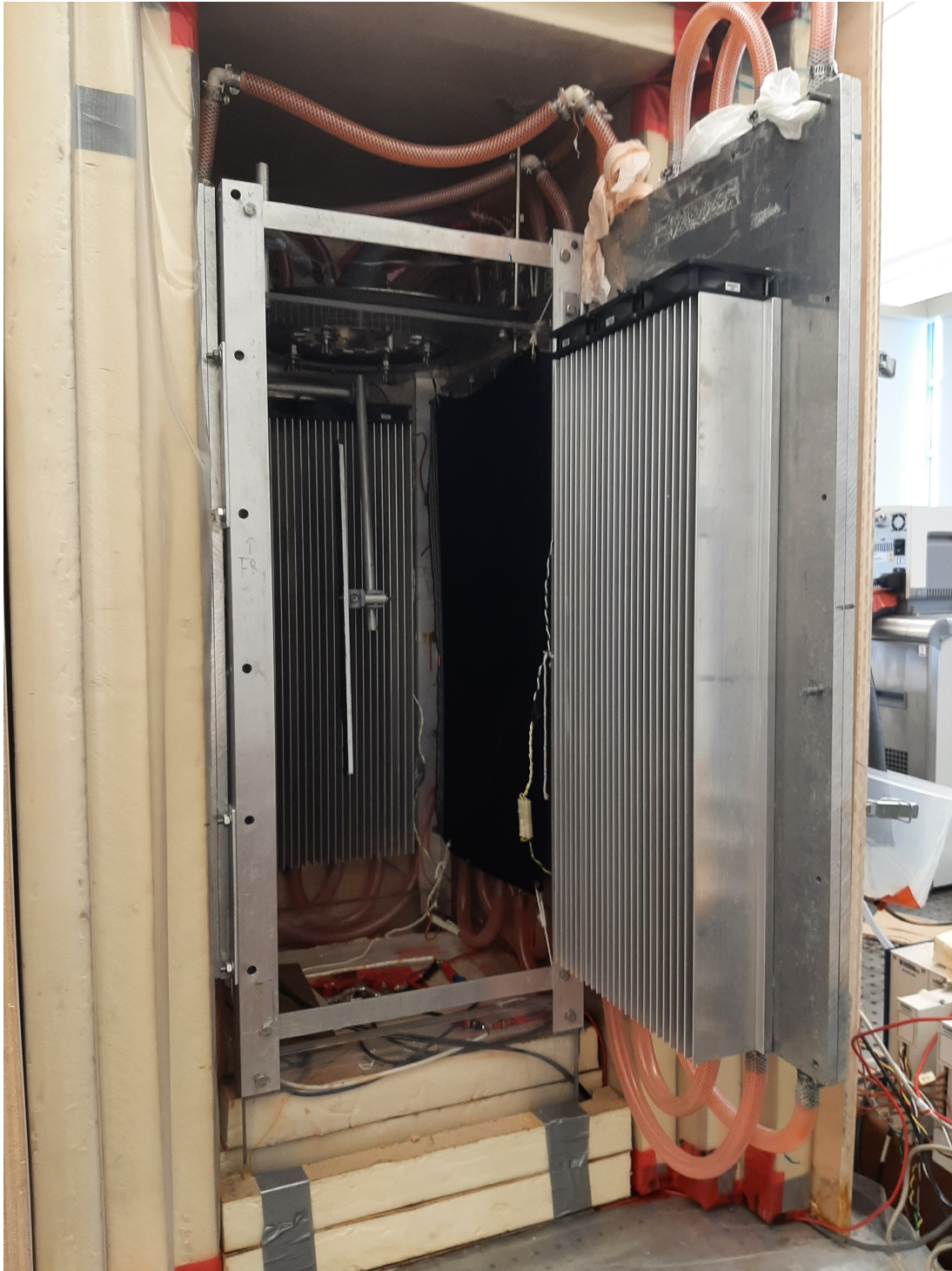
Figure 3.3: A close-up of the icicle chamber interior. The interior aluminum walls form a frame to hold the lighting, thermocouples, and rotating icicle support. The interior walls are cooled with antifreeze that circulates through them. The open door has one set of circulating fans and a heatsink, with the other fans and heatsink attached to the opposing wall. Black velvet is suspended by four corners at the back of the chamber to provide a contrasting background.
