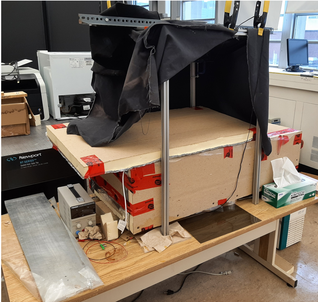
Figure 3.13: The refrigerated box and camera frame used to take pictures of sectioned icicles. The aluminum plate used to create the sections is shown to the left of the box.
