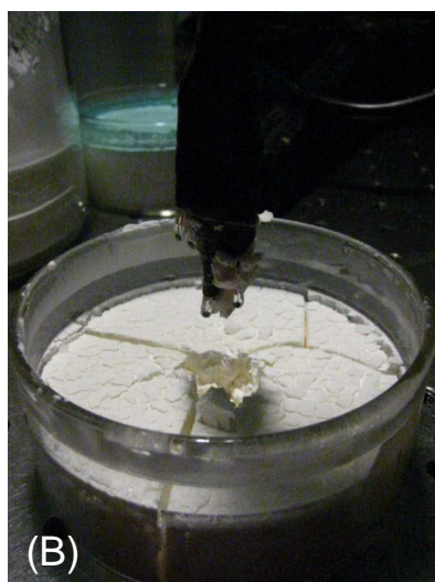
Fig. 2.3 Temperature investigations. (A) Temperature within a starch plug is seen to be dependant on time and depth. (B) Thermal probe, as just removed from a dried sample. (C) Calibration fit of a thermistor.
