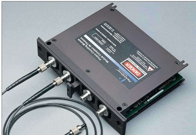
To avoid a degradation of the module linearity and stability, the heat sink temperature should be kept between 5°C and 40° C during operation.
