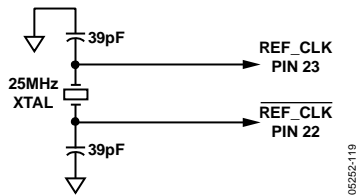
Figure 35. Crystal Input Configuration
