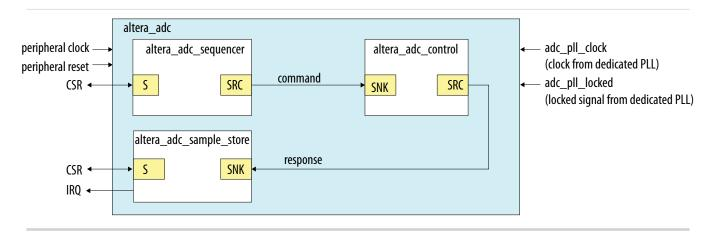
Figure 2-8: Standard Sequencer with Avalon-MM Sample Storage (Altera Modular Dual ADC IP Core)
