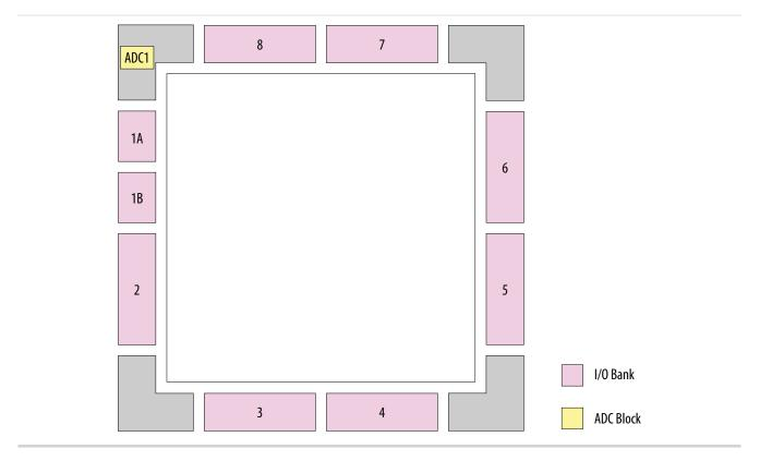
Figure 2-3: ADC Block Location in MAX 10 16 Devices
