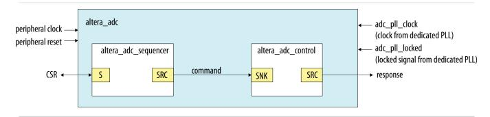
Figure 2-12: Standard Sequencer with External Sample Storage (Altera Modular Dual ADC IP Core)
