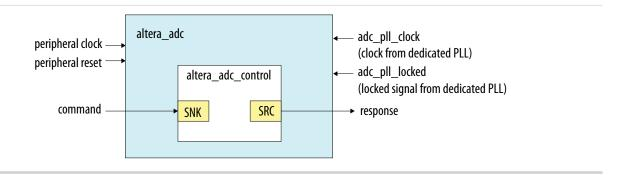
Figure 2-14: ADC Control Core Only (Altera Modular Dual ADC IP Core)
