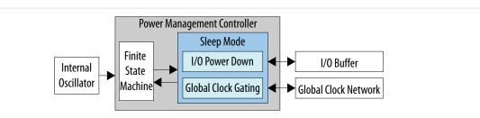
The MAX 10 device contains hardware features that enable I/O power down and global clock (GCLK) gating to manage low-power state during sleep mode. You can power down the I/O buffer dynamically when your application is in idle or sleep mode. One example is the digital single lens reflex DSLR camera
