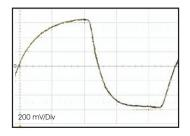
Note: The clipped sinewave output is AC coupled
