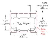
\* Do not route any traces in the keep out area. It is recommended the next layer under the keep out area is to be ground plane.
