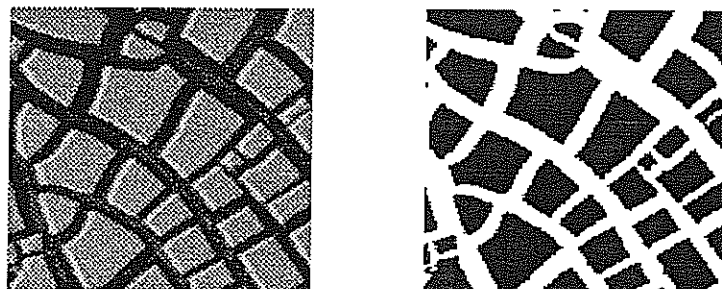
Figure 3.8: Greyscale and black and white images of an 8 cm \times 8 cm region of the crack pattern for a Type B experiment with d = 2.64 \pm 0.09 mm.
