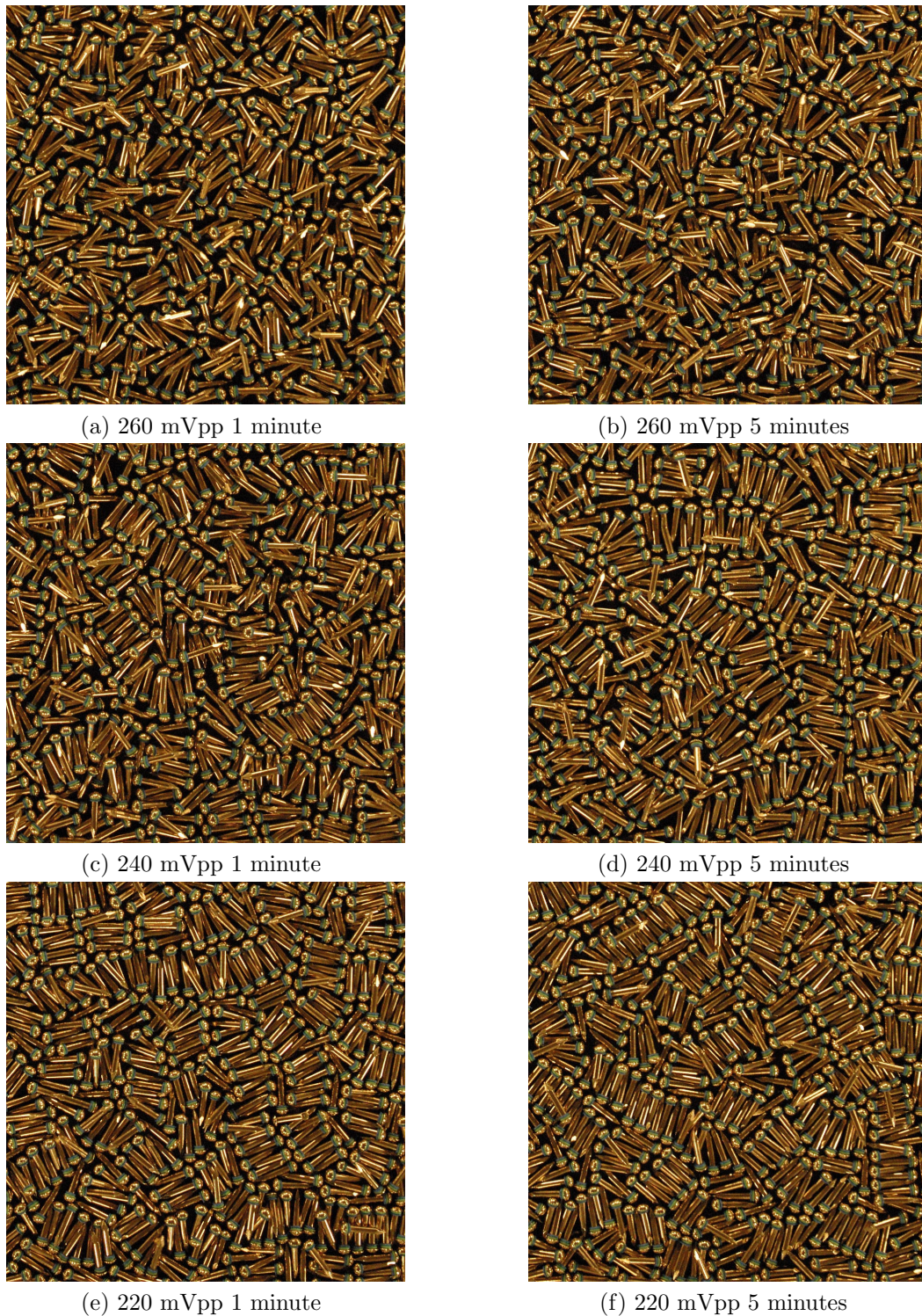
Figure 3.3: Examples of the experiment with 1/2 inch nails at 95.7% packing fraction to determine if time was a factor in antiferromagnetic ordering, as outlined in the text. Images are cropped to 1/4 of the plate area in order to show detail.
