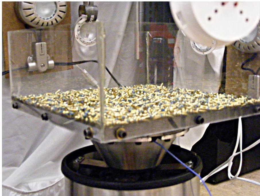
(b) Side view of the shaker plate, showing the barrier walls and circular cone.
