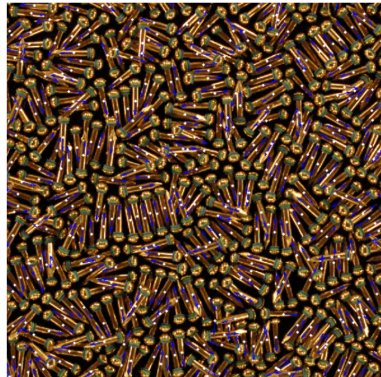
(c) Nails that have been detected using tagging, after first edit.
