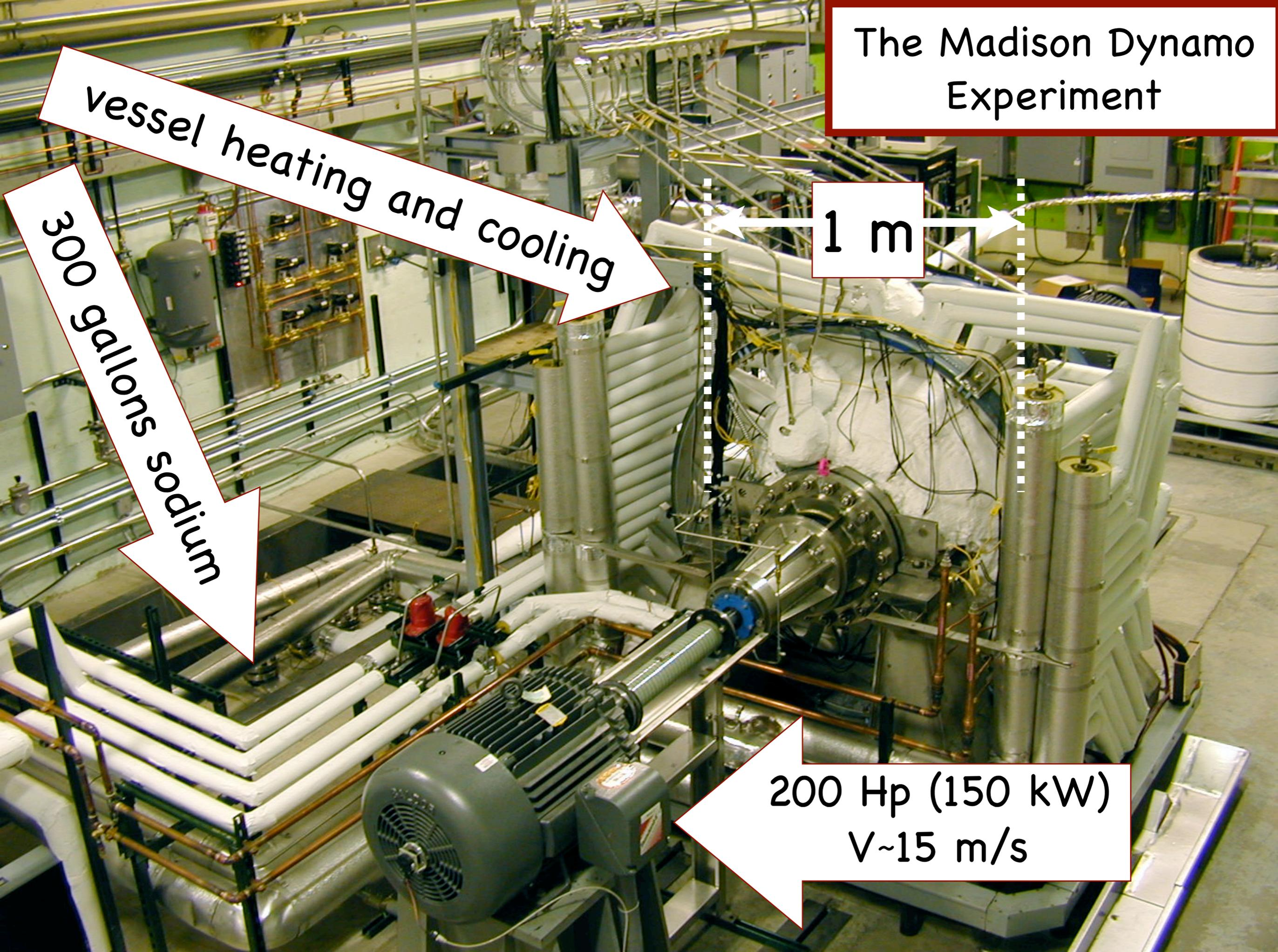
Magnetic field is measured both internally and externally;
