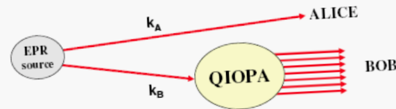
FIG. 1: Schematic diagram showing the single photon Quantum-Injected Optical Parametric Amplification (QIOPA).
