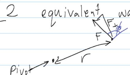
2 equivalent ways of computing torque.
