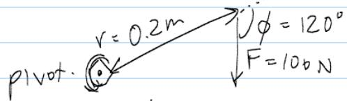
$$\begin{aligned} |\tau| &= |r F \sin \phi| \\ &= (0.2)(100)(\sin 120^\circ) \\ |\tau| &= 17.3 \text{ N}\cdot\text{m} \end{aligned}$$
