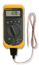
photo is  $0.4^{\circ}$ C. It means one-half of the power of ten represented in the last digit. Here, the last digit represents values of a tenth of a degree, so the reading error is  $1/2 \times 0.1 = 0.05^{\circ}$ C. You should write the temperature as  $12.80 \pm 0.05^{\circ}$ C.
