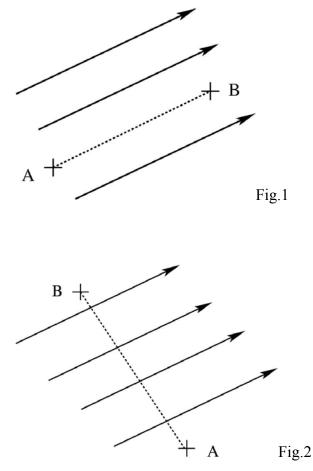
Thus, the electric field does no work on the charge q as it moves from point A to point B. Since no force resists the motion along the path, we are free to imagine that virtually any small force whatever could have moved the charge q along this path; the cause of this force is irrelevant. The point here is that the electric field does no work on any charge moved along a path that is everywhere perpendicular to the electric field.
