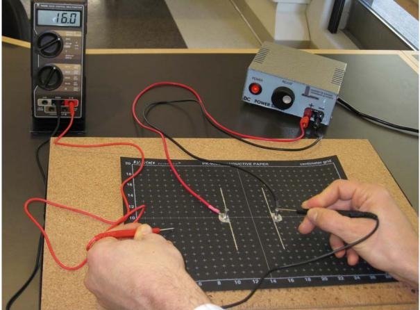
10. Gently scrape the red probe over the paper between the two objects until you find a point at which the potential (voltage) is about 5 Volts; <u>don't make any pencil or pen marks on the black paper</u>. Next, find the path from this point along which the potential stays constant at 5 Volts; follow this path wherever it leads, even if the path curves around behind the edges of the objects. This path
