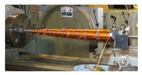
**Figure 3.4.:** The Zeeman slower after winding in the lathe of the machine shop. The begin and end of each layer is tightened with a hose clamp (1); moreover, the teflon holder (2) straightening the wire and giving control about its position as well as the stopper wheel (3) is shown.
