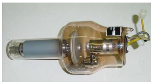
**Figure 5.** A typical rotating anode x-ray tube.
