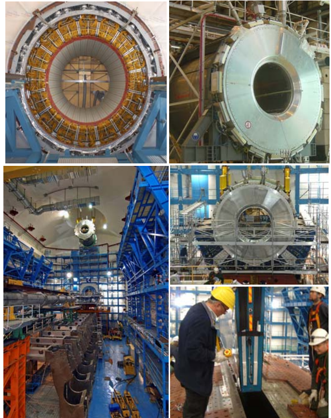
Fig. 7. Top: View of the ATLAS EMB calorimeter installed in the Barrel Cryostat. The pre-sampler is visible inside the calorimeter. The right-hand photo shows the completed cryostat. The pedestals for the Front End Crates are visible around the periphery. Below: View of the ATLAS Barrel Cryostat being lowered into the ATLAS Cavern at LHC Point 1. The cryostat is lowered onto the partially assembled Tile Calorimeter, the construction of which is then completed around it (lower right).
