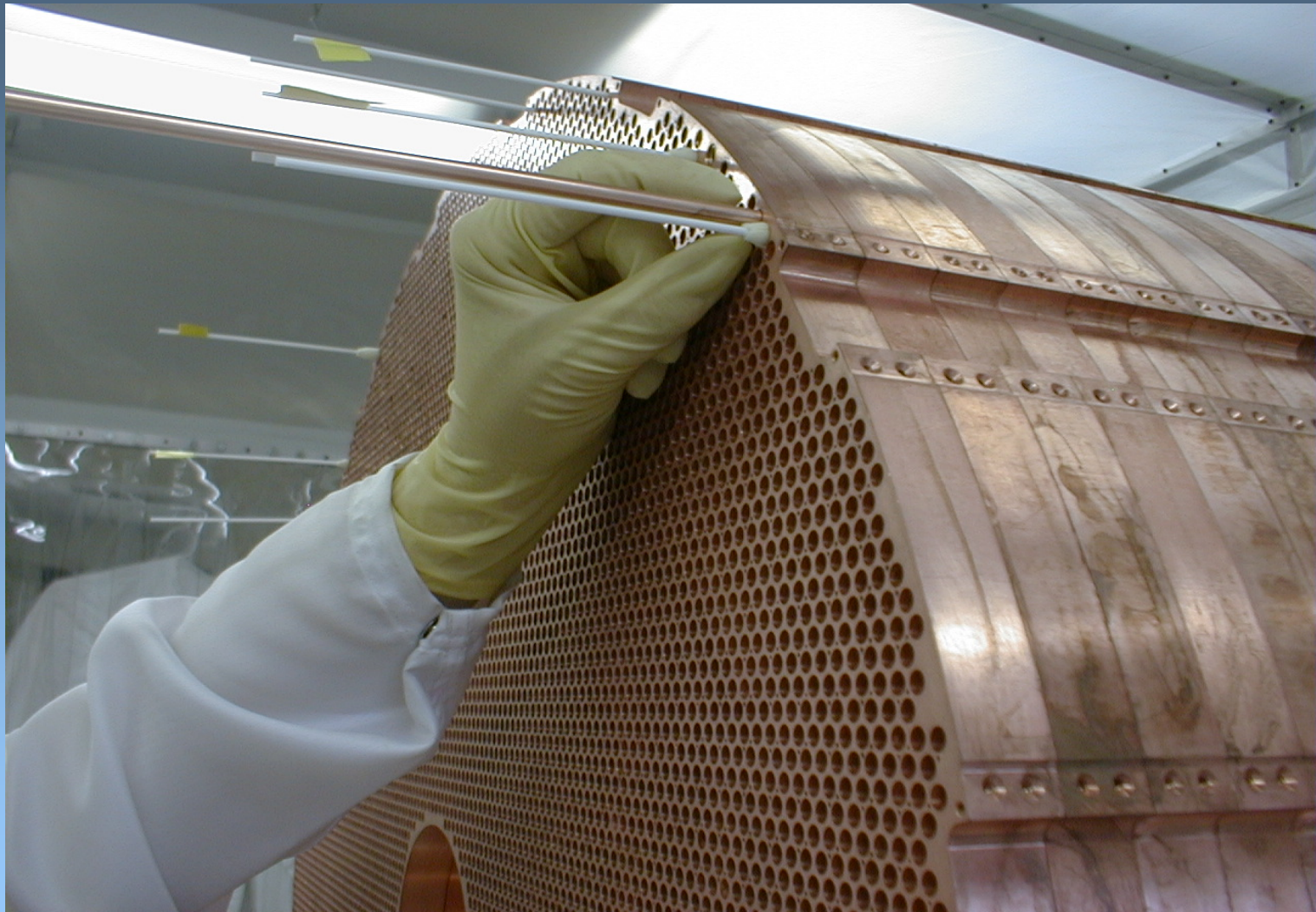
Insertion of FCal1 electrode tube
