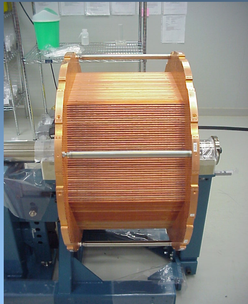
During matrix stacking (tubes and slugs)
