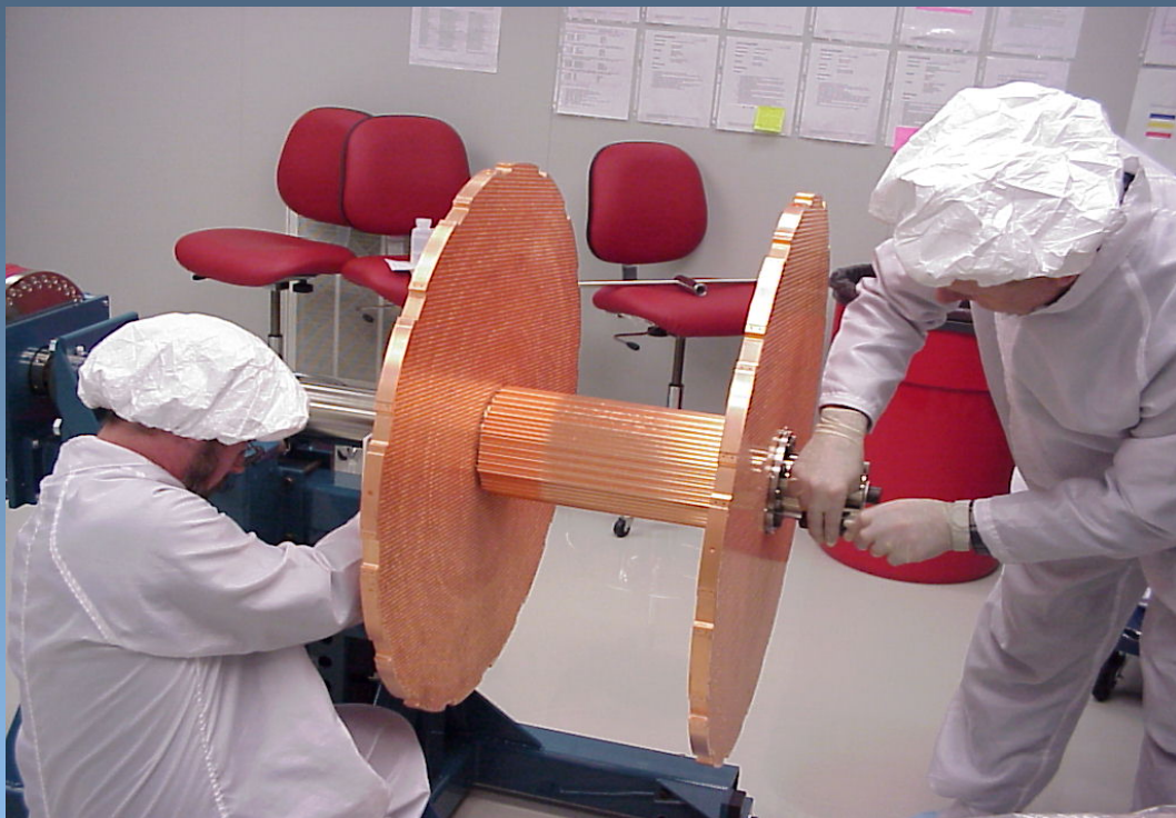
Endplate and inner absorber assembly
