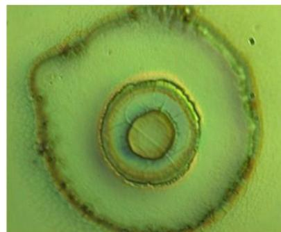
**Figure 14.**  $10\ \mu\text{s}$  laser pulsetrain at threshold fluence, on broadband  $1280 - 1600\text{nm}$  HR mirror. Clean removal of dielectric layers, some material modification on perimeter of site, and slight thermal-shock fracturing due to long-time post-train leakage. Image has been both top-illuminated and also viewed through a single polarizer.
