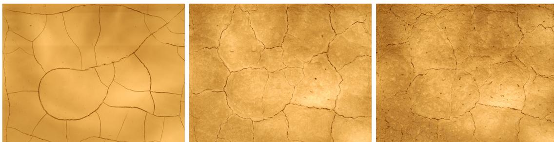
Figure 5: Left: a cropped image of the third crack pattern, just before re-wetting. Middle: The same pattern after 50 cycles, and right: after 152 cycles.
