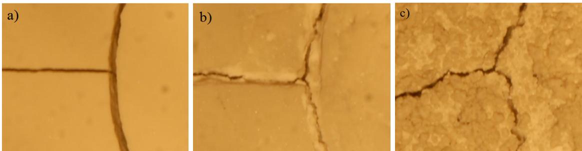
Figure 6: Vertex at the middle-left of the curved ped, for a) 1 cycle, b) 29 cycles, and c) 102 cycles.
