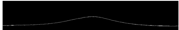
FIG. 3: Visualization of the edge data describing the location of the water's surface obtained from FIG. 2
