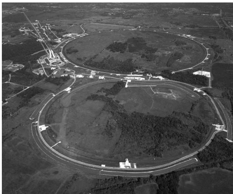
Figure 3. Aerial view of the Fermilab accelerator complex. The initial proton acceleration and antiproton production takes place at the top left of the picture. Different accelerators in the near ring cool the antiprotons and ramp both proton and antiproton beams to 150 GeV prior to Tevatron insertion. The ring in the distance is the 6.28 km circumference Tevatron collider. The 980 GeV beams are brought together to collide at two points where experiments are sited (photograph courtesy of Fermilab VisualMedia Services).
