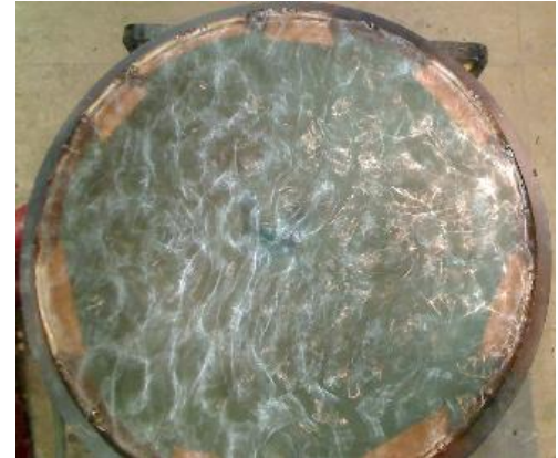
FIG.4: Stable pattern on the water surface. h = 1.2 cm; f = 20 Hz; \Gamma = 0.15
