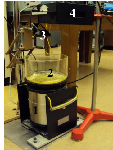
FIG.1: 1 – shaker; 2 – vessel with fluid; 3 – digital camera; 4 - stroboscope
