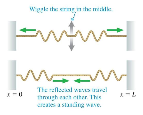
Reflections at the ends of the string cause waves of equal amplitude and wavelength to travel in opposite directions along the string, which results in a standing wave.
