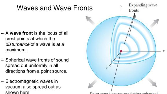
Point sound source producing spherical sound waves (alternating compressions and rarefactions of air)
