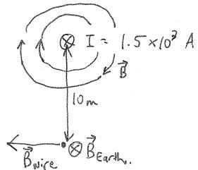
$B_{\text{Earth}} = 0.24 G = 2.4 \times 10^{-5} \text{ T}$   $B_{\text{wire}} = M_0 I = \frac{4\pi \times 10^{-7} (1.5 \times 10^3)}{2\pi r}$
