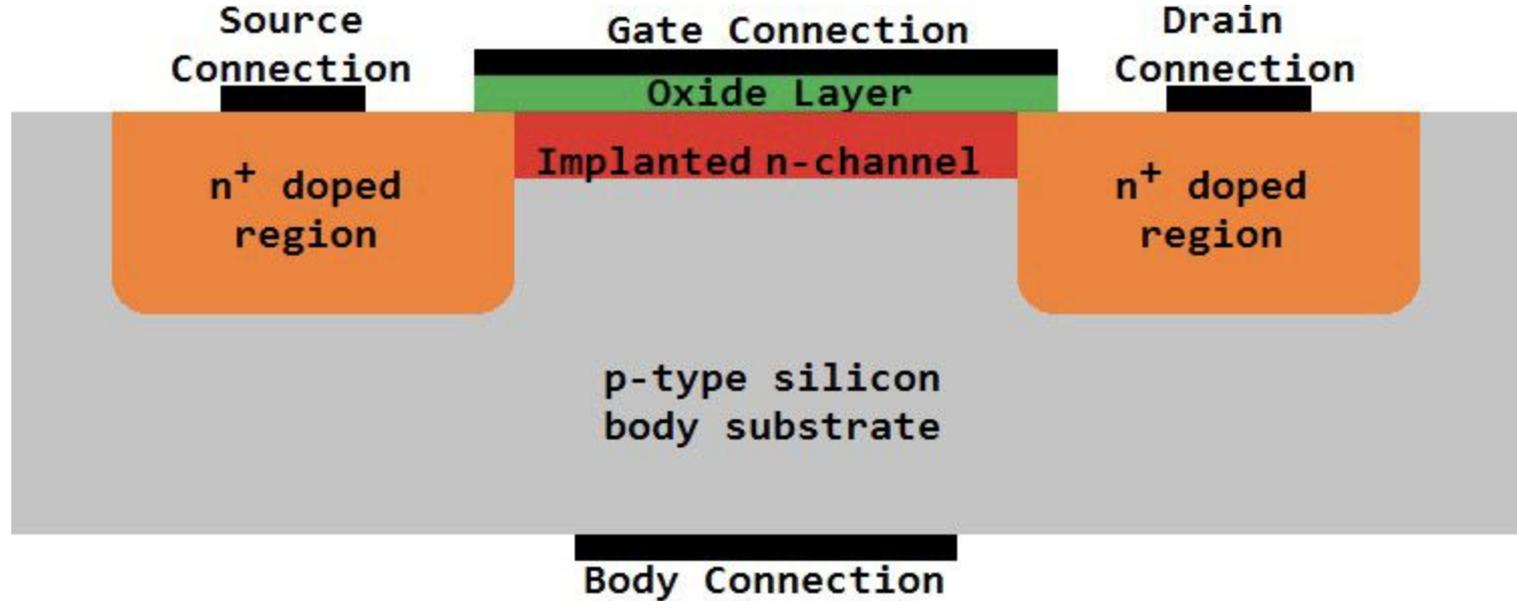
n-channel depletion-mode MOSFET. Current can normally flow through the n-type connection between Source and Drain. (source: [DigiKey](#)).
