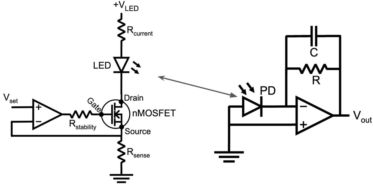
Control  $V_{set}$  with Arduino digital pin, detect LED output with photodiode, observe signal on scope
