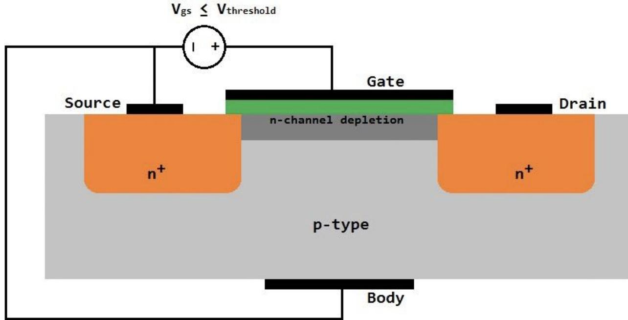
Current is blocked when a negative Gate voltage repels electrons from the connection, turning it effectively into p-type. (source: [DigiKey](#)).
