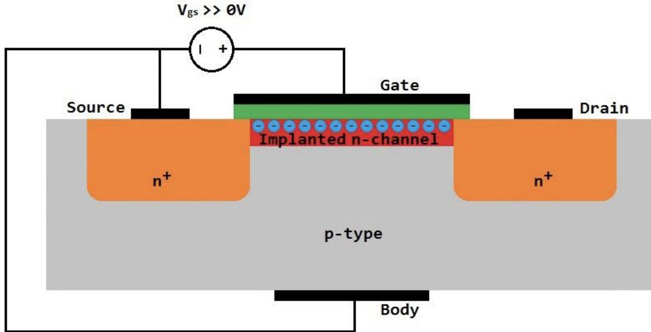
Current increases when positive gate voltage attracts electrons and enhances the conduction channel. (source: [DigiKey](#)).
