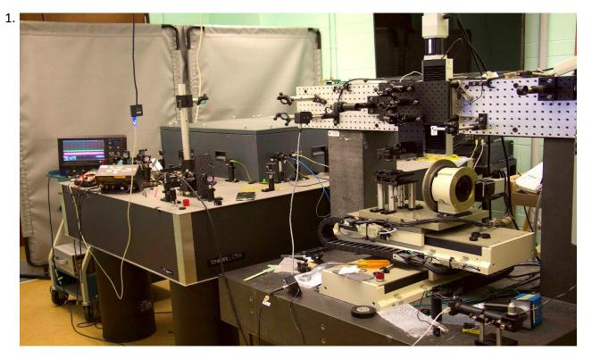
Photo 1: Our new compact and robust burst-mode ultrafast fiber laser gives us new capabilities for applied physics studies of materials-processing using femtosecond laser pulses in 200MHz 'bursts' of pulses. New methods of making microfluidic structures, treating strengthened glass, processing new forms of condensed matter, specially treating high-value crystals and others are examples of the ways that new physics approaches can have a big impact on R&D in industry
