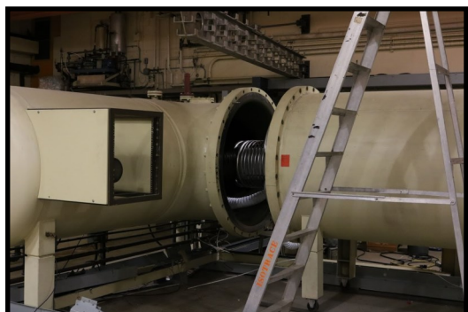
The 3 MV power supply tank (right side behind the ladder) separated from the accelerator tank (left). Photo Credit: Victoria Fisher
