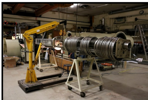
Removing the equipotential rings from the accelerator column. Photo Credit: Victoria Fisher
