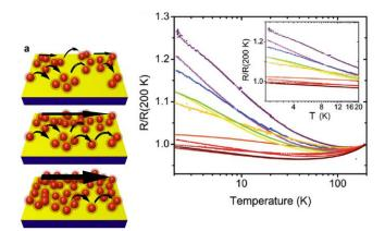
Some recent results from the Dhirani group. Left panel. Self-assembling nanoparticles into films. Right panel. At lower temperature, films exhibit a large, log increase in resistance due to quantum hybridization between delocalized electrons and localized electrons with unpaired spins in quantized energy levels.
