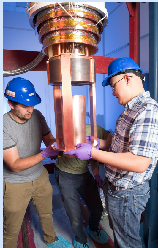
Noah Kurinsky (left), Ziqing Hong (right) and Brian Nebolsky (in the back) installing a SuperCDMS-type detector at a SuperCDMS test facility.
