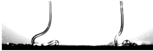
Figure 35: Buckling of thread causing discontinuity in position of point of contact
