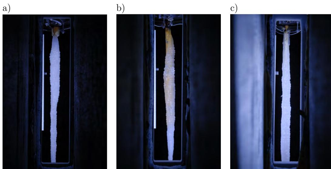
Figure 2.3: Examples of Icicles grown on a) the small conical support, b) the sham-wow stick, and c) the wool stick)
