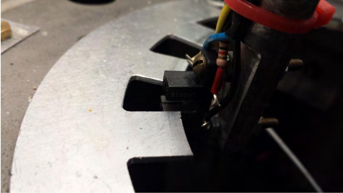
Figure 2.4: Image of the interrupter as it passes through a tab on the rotating ring, blocking the interrupter beam. When the beam is interrupted the LabVIEW VI is programmed to take a picture.
