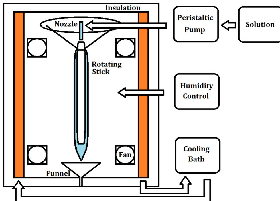
Figure 2.2: Schematic diagram of the apparatus, including the box in which icicles are grown along with external tools such as the peristaltic pump and humidity control.
