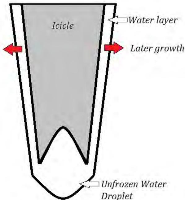
Figure 1.1: Drawing depicting the mechanism of icicle growth
