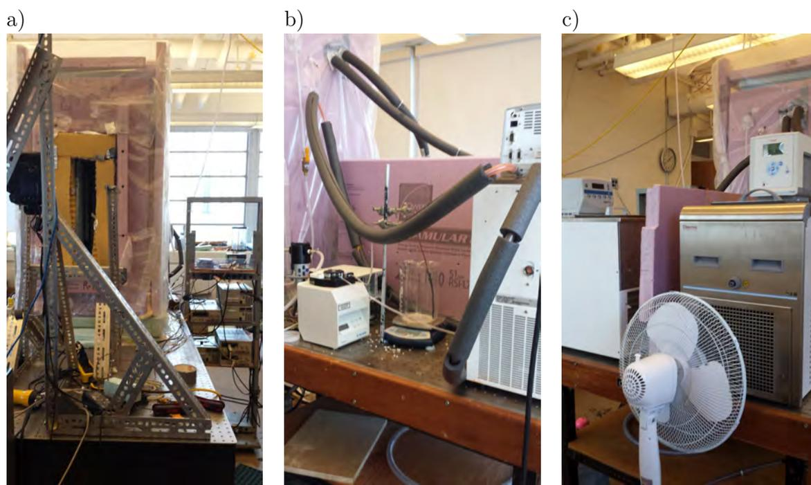
Figure 2.1: a) Image of the front of the icicle growth apparatus. b) Image of the side of the apparatus, including the peristaltic pump, mass balance and humidity regulator. c) Image of the back of the apparatus, including both of the cooling baths.
