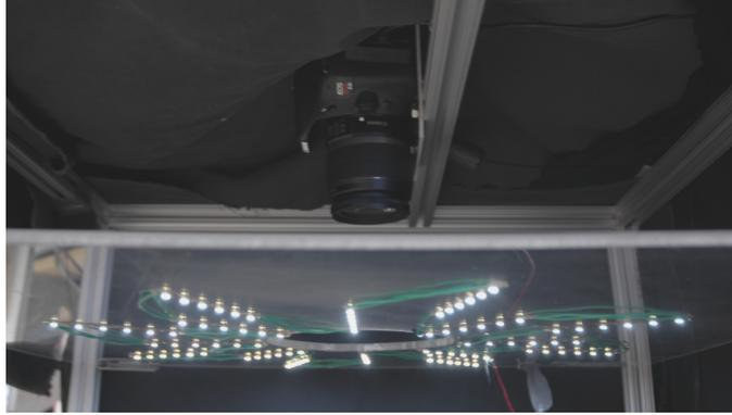
Figure 2.2: Canon Rebel T2i and LED array used to capture images of shaking chains.
