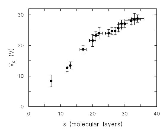
FIG. 3. The onset voltage  $V_c$  as a function of film thickness for films 20.0 mm by 2.0 mm.
