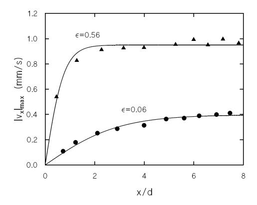
FIG. 9. The maximum value of  $|v_x|$  in each vortex as a function of distance from the sidewall for two values of  $\epsilon$ . The curves are fits of Eq. 1.3 to the data. The film had dimensions 10.0 mm by 0.66 mm and was 3 molecular layers thick.
