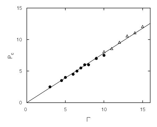
FIG. 5. The number of vortex pairs at the convective onset  $P_c$  as a function of aspect ratio  $\Gamma$ . The open triangles were measured on films 1.0 mm wide, and the solid circles on films 2.0 mm wide. The solid line is a linear fit through the origin to both sets of data.
