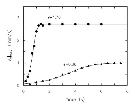
FIG. 11. Evolution of the velocity amplitude after a sudden change of the voltage across the film from zero to a supercritical value. The curves are fits of Eq. 1.5 to the data. The film thickness was 20 molecular layers.
