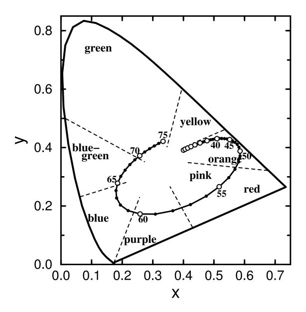
FIG. 2. The calculated colour of 8CB films illuminated by a CIE standard source A at normal incidence, plotted on a CIE chromaticity diagram. Here the axes are CIE chromaticity coordinates, and the numbers on the diagram give the film thickness in molecular layers.
