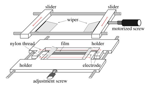
FIG. 1. Diagram of the film holder used in the experiments.
