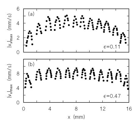
FIG. 8.  $|v_x|$  as a function of position along the length of a film for two values of  $\epsilon$ . Convection is suppressed near the end walls. The film had dimensions 16.0 mm by 2.0 mm.
