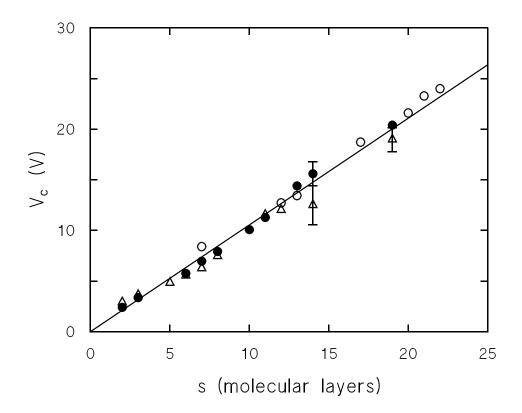
FIG. 4. Onset voltage as a function of film thickness for very thin films of three different sizes. Solid circles: 10.0 mm by 0.7 mm; open circles: 20.0 mm by 2.0 mm; open triangles: 15.0 mm 1.0 mm. The line is a fit through the origin to all of the data.
