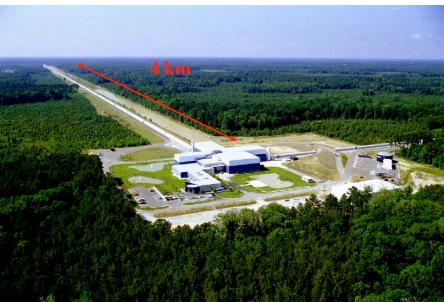
The arms are empty vacuum - all that matters is the motion of the mirrors on the end. They are suspended like little pendulums, to be immune as much as possible from earthquakes, logging, trucks,...
