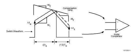
FIGURE 3. Compensation Ramp Avoids Sub-Harmonic Oscillation
