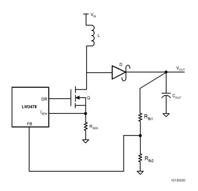
FIGURE 10. Adjusting the Output Voltage
