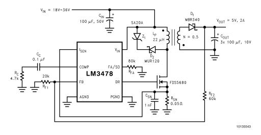
FIGURE 13. Typical Flyback Circuit
