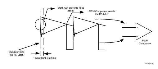
FIGURE 1. Basic Operation of the PWM comparator
