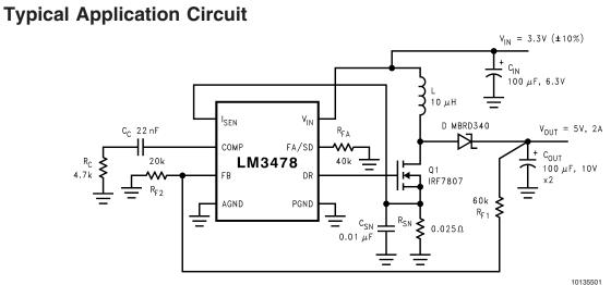
Typical High Efficiency Step-Up (Boost) Converter
