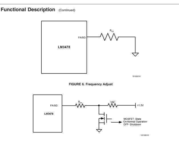
FIGURE 7. Shutdown Operation in Frequency Adjust Mode
