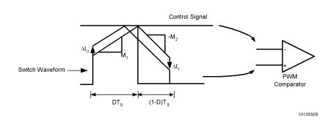
FIGURE 2. Sub-Harmonic Oscillation for D>0.5
