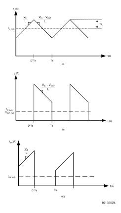
FIGURE 9. A. Inductor current B. Diode current
