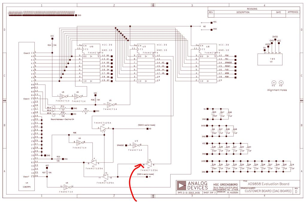
BUG! Lift U1.8 and insert 1K in series. This allows use of the U4 pin header as a parallel input, such as the Rabbit RCM3200 module.
