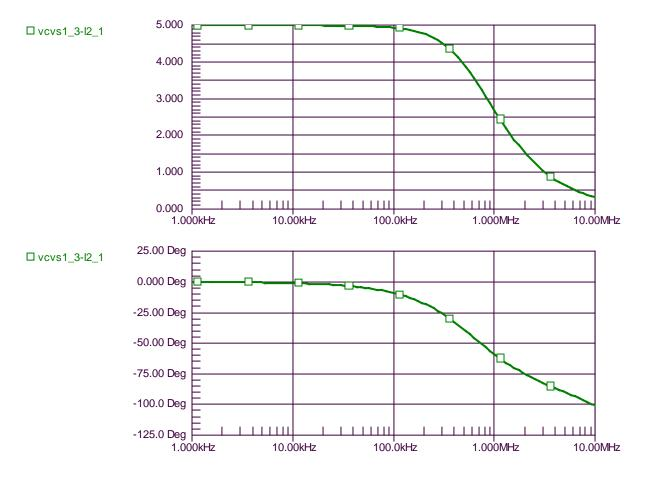
However, the disadvantage of the sense-resistor zero is also evident. While the response is flat and stable the bandwidth is significantly reduced, from over 1 MHz to somewhat above 600 kHz. Can bandwidth be extended while retaining a flat magnitude response? A faster forward-path amplifier will not extend bandwidth much because of the sense-R zero, which appears as a pole in the closed-loop response. But by using a lower-
