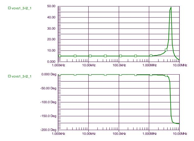
Now, introduce a realistic value of 50 nH of parasitic series inductance for a twoterminal, 5 W, 0.2  $\Omega$  sense resistor. The forward-path amplifier is modeled as an ideal (infinite bandwidth) amplifier, U<sub>1</sub>, followed by a single-pole roll-off RC circuit (R3, C2) and an ideal ×1 buffer amplifier. The overall forward-path model is one of a voltage amplifier with a single pole. For large U<sub>1</sub> static (dc) gain, the closed-loop gain is approximately:
