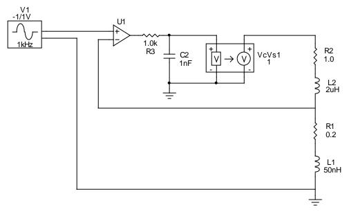
The load inductor,  $L_2$ , is modeled as a series RL with the addition of  $R_2$ . The sense resistor model is also a series RL,  $R_s$ ,  $L_s$ , shown as R1 and L1 in the circuit diagram. To amplify current a voltage proportional to output current is fed back from the sense resistor. The resultant RL sense-resistor combination has an impedance of:
