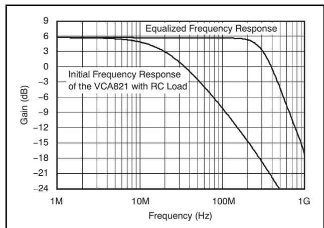
Figure 78. Differential Equalization of an RC Load
