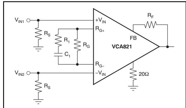
Figure 77. Differential Equalizer
