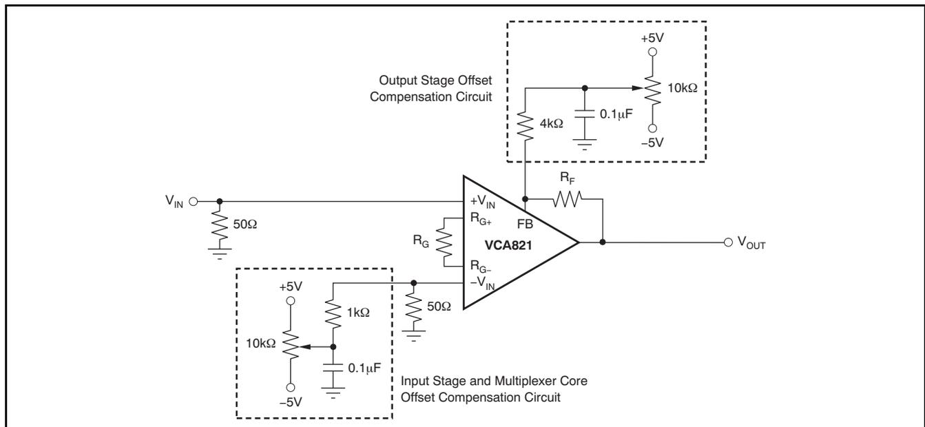
Figure 85. Adjusting the Input and Output Voltage Sources
